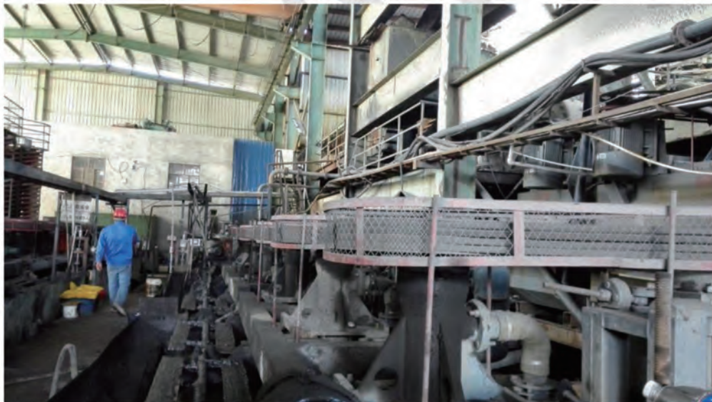
Figure 10-7 Flotation circuit of the Baicao Processing Plant
