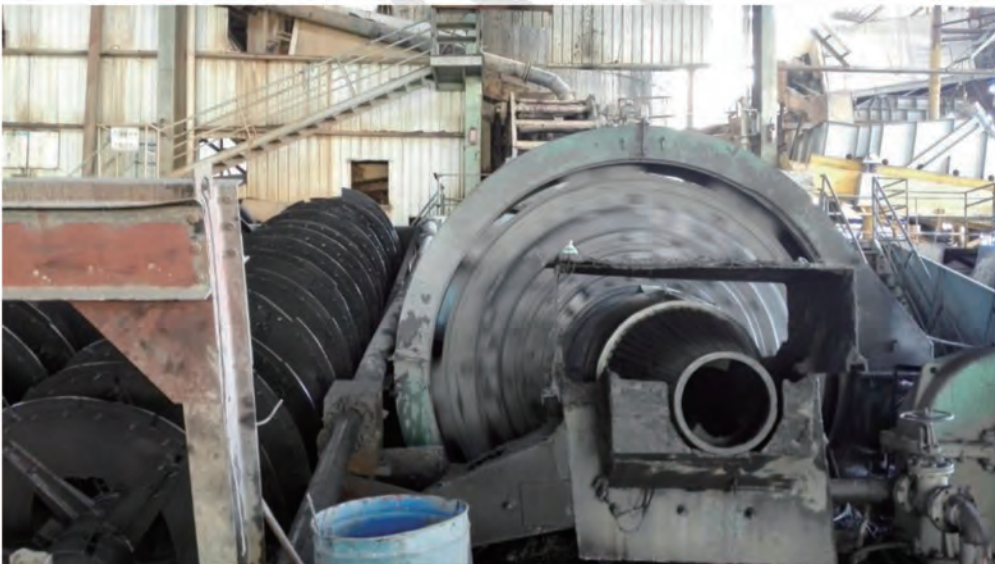
Figure 10-5 Ball mills of the Baicao Processing Plant
