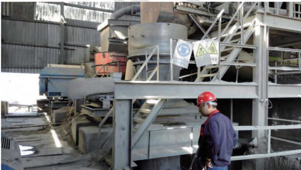
Figure 10-3 Secondary crusher of the Baicao Processing Plant
